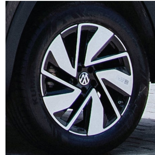
20" Atlanta Alloy Wheel (8J x 20) with 255/50 R20 tyres (Standard on the Teramont)
